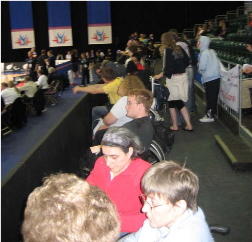
Picture showing poor circulation space provided for wheelchair users, restricting access to exits and toilet facilities
